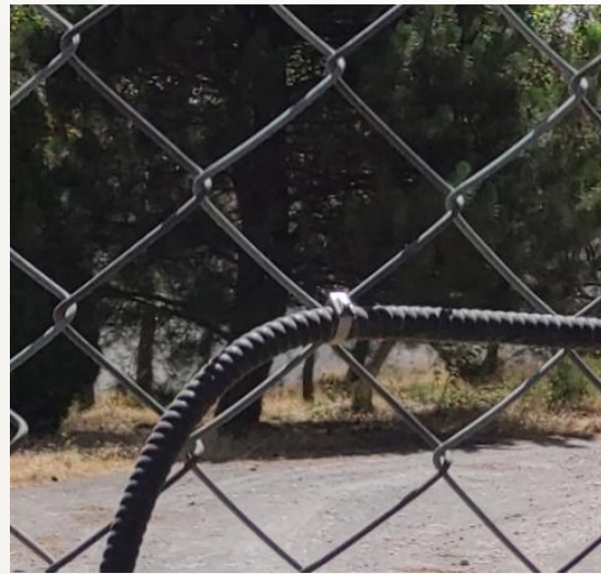
Armored microphonic cable with cable tie for connecting the cable to fence
